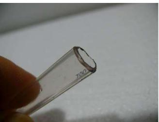
You can also wet the tip of the tube, hold the tube tilted, so one side is in the opening and then push in the other side (this requires some force.)
