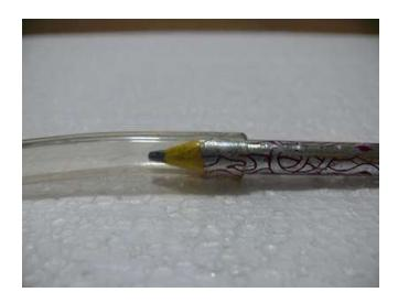
To get the tube onto the pump outlet, widen it by heating the tube material with the flame of a lighter (be sure not to burn it) and then pushing a pencil into the opening when the tube end is still hot and soft. It will then slip onto the pump easily.
